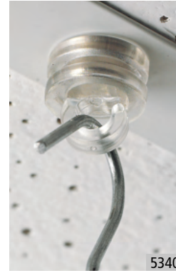
MINI MAGNETIC CEILING LOOP Clear polycarbonate encased neo magnet with 6mm Ø closed loop. Supports loads pull up to approx 1.2kg 5341 16mm Ø
