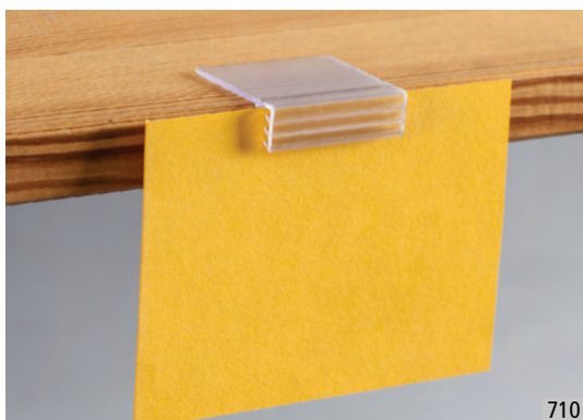
SHELF EDGE FLUSH SIGN HOLDER Clear co-extruded PVC Supergrip. Fits shelves 8-15mm thick. Holds material up to 2mm thick 710 38mm long
